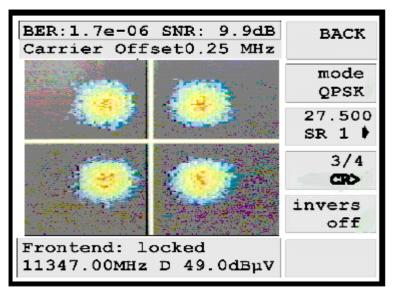
For the digital transmission via satellite, the modulation type QPSK (Quadrature Phase Shift Keying) is used. Every 2 information bits are put together to one symbol and modulate one carrier in its phase. With this, four conditions are possible, which a receiver must recognise.
